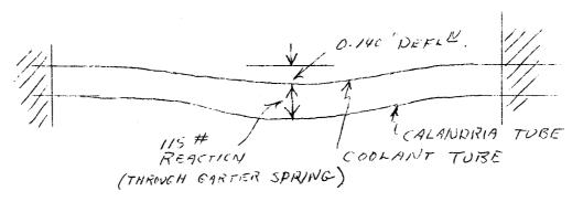
The calandria tube takes part of the weight of the coolant tube through the garter spring space. The total coolant tube, calandria tube deflection is calculated to be 0.140 inches.
